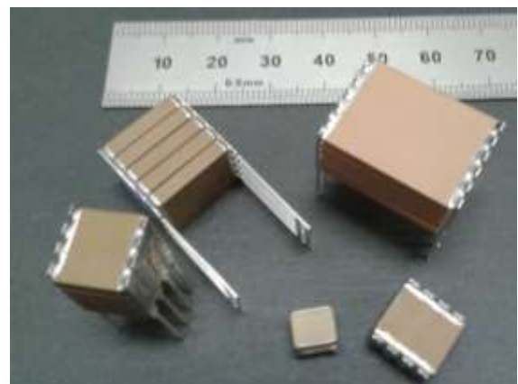
Fig 2. Various stacked assemblies up to 8060 5 stack
