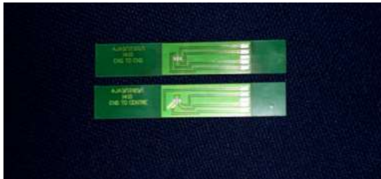
Example of FR4 Test PCB Used
