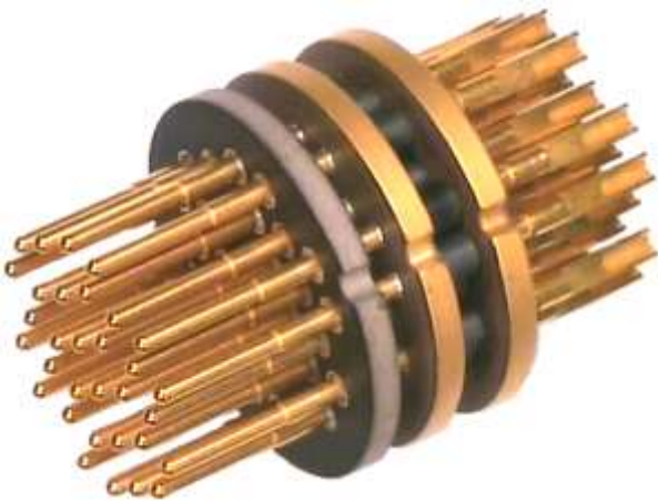
Fig. 6 The internal configuration of a varistor protected unbalanced Pi
