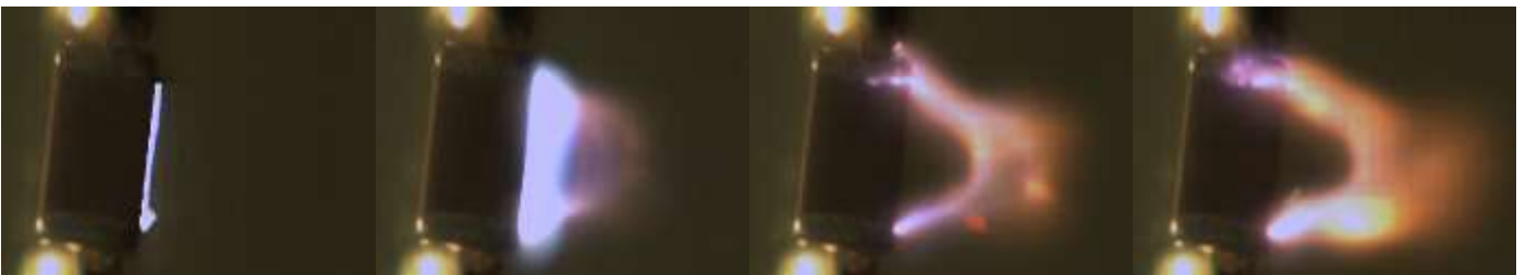
Pictures showing the propagation of surface arc.
