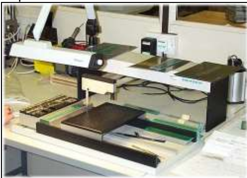
Hand pick and place used to mount capacitors for bend tests
