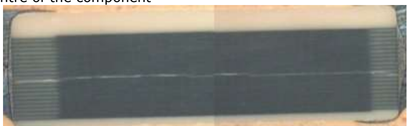
Fig 7. Piezo stress crack failure
